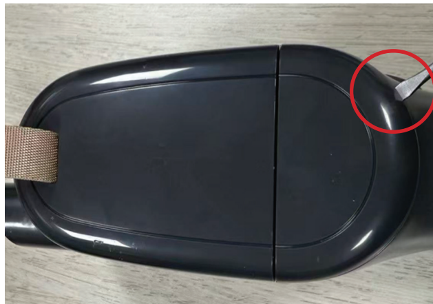
10. Remove the left cover plate using a flat-head screwdriver (or any other suitable tool)
