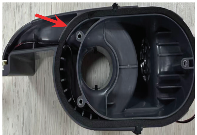
28. Remove the cyclone eva sealing
