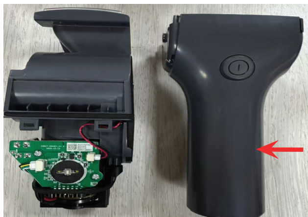
18. Remove the filter mesh frame
