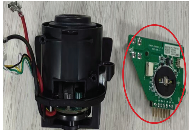
24. Remove the button-PCBA
