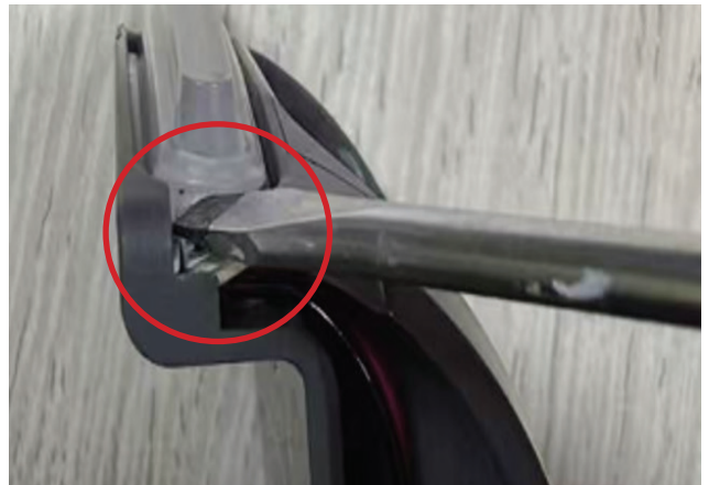
28. Remove the cyclone eva sealing
