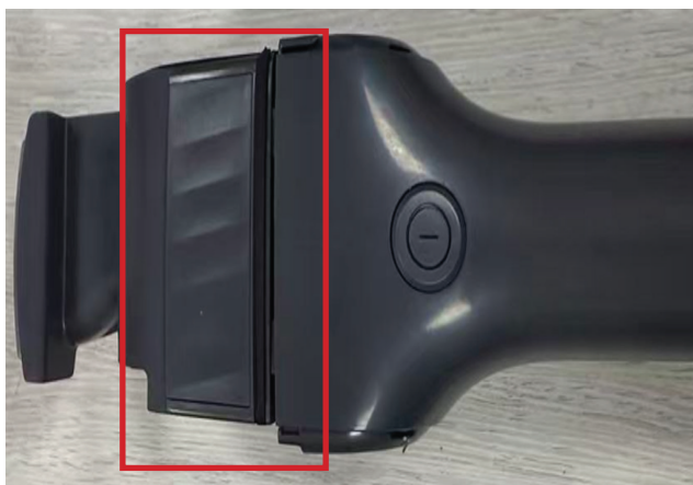
15. Remove the cyclone assembly
