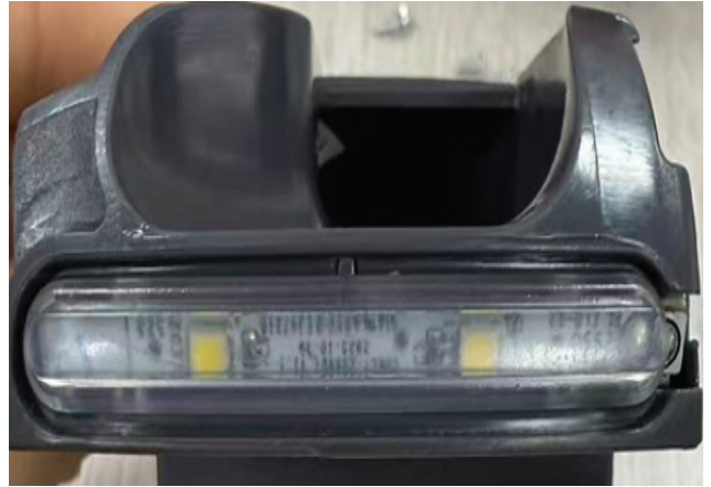
27. Remove the lampshade using a flat-head screwdriver (or any other suitable tool)
