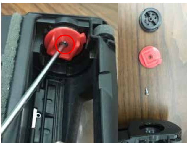
19. Remove two front wheels, dismantling two snaps and eight screws to dismantling the bottom base.
