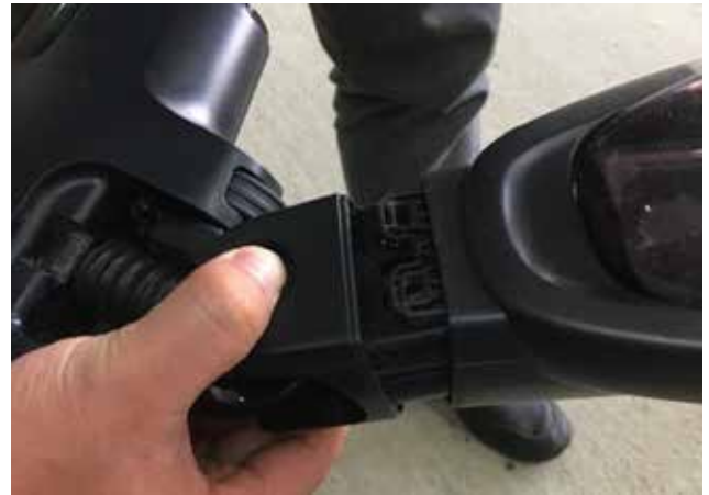
24. Remove right cover, take down the brush bar, unscrew two screws of the left cover, then take down left cover.
