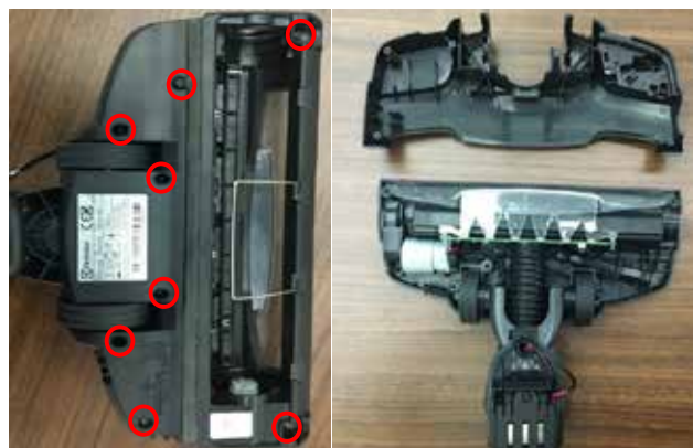
20. Dismantling other components from base.
