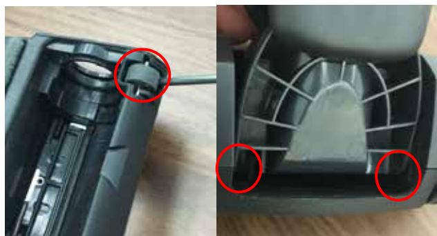
19. Remove two front wheels, dismantling two snaps and eight screws to dismantling the bottom base.
