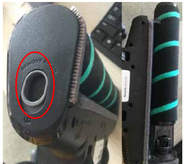
24. Remove right cover, take down the brush bar, unscrew two screws of the left cover, then take down left cover.
