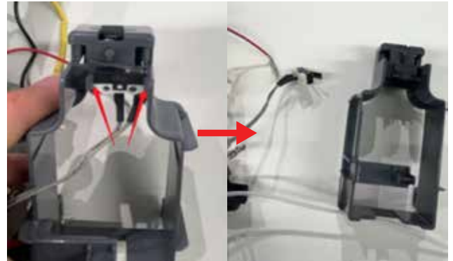
37. Release the wire protection part (rubber part)
