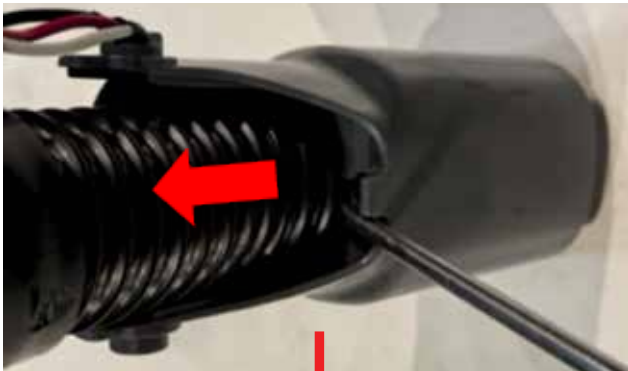
62. Release hose overmold assembly
