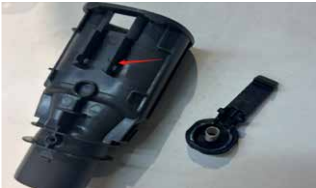
08. Release tube release button spring
