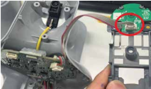
45. Remove the light guide and rubber part
