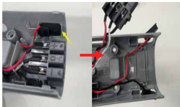
25. Releasing the charging contact in the front in both side
