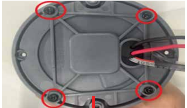
41. Remove four screws in the motor housing
