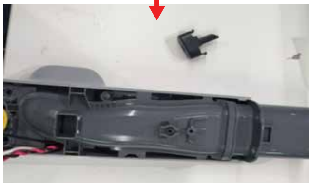
24. Pushing the snap and release the air channel assembly
