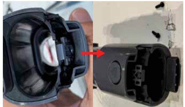
66. Push nozzle release button and then pull out, release the upper connector inside lining
