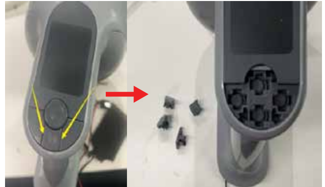
36. Releasing the two screws
