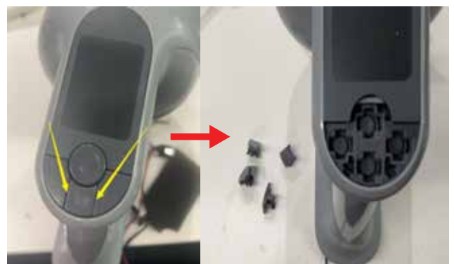
38. Releasing the four buttons and screen
