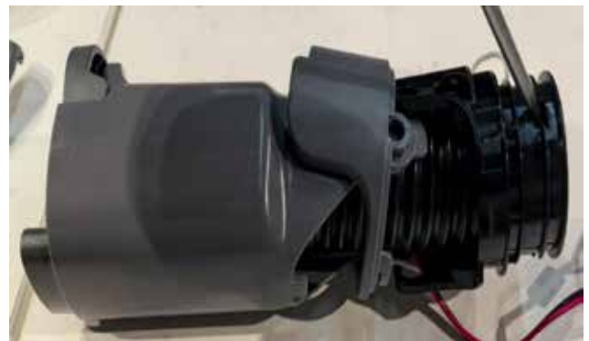
57. Release lower connector inside lining
