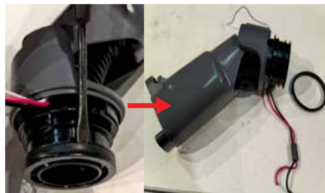
53. Release lower connector seal
