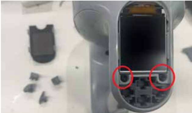
40. Releasing the housing and depart the motor housing assembly
