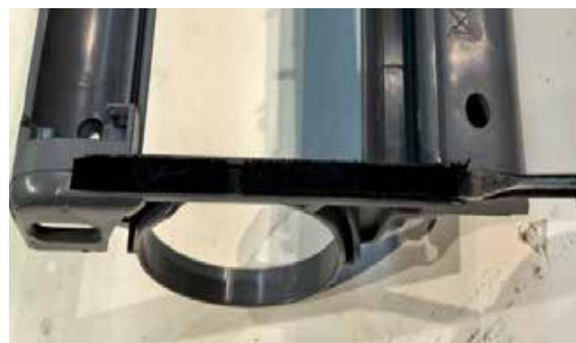
53. Release lower connector seal
