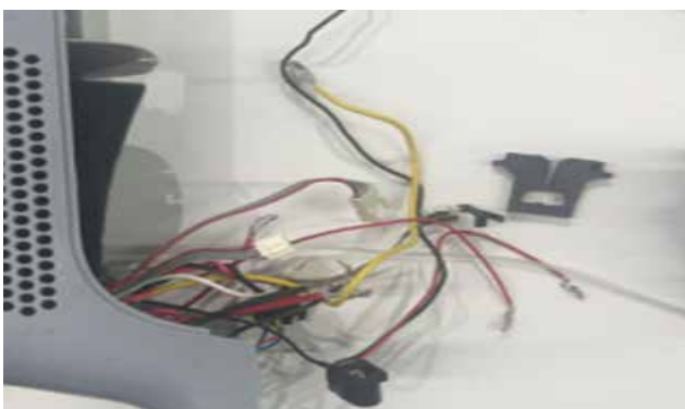
34. Releasing the wire protection part(rubber part)
