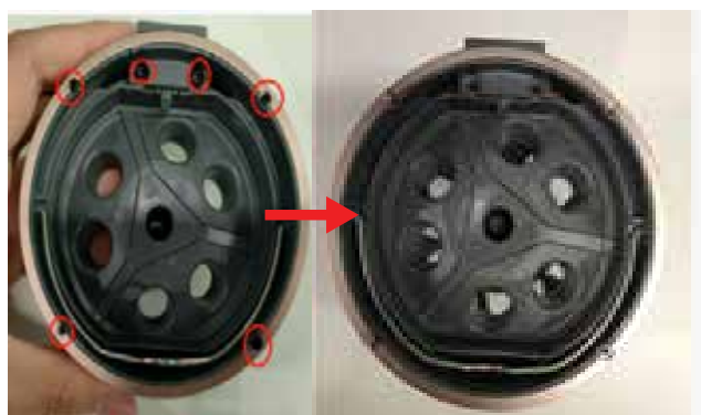
6. Releasing six screws
