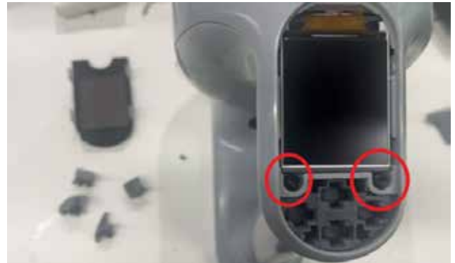
37. Releasing the housing and depart the motor assembly from it
