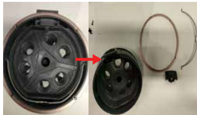
8. Rotate the upper area and depart the cyclone assembly
