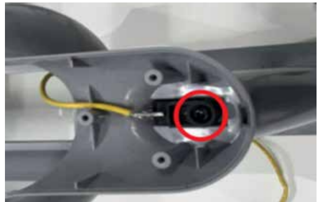
47. Remove the screw for ESD releasing
