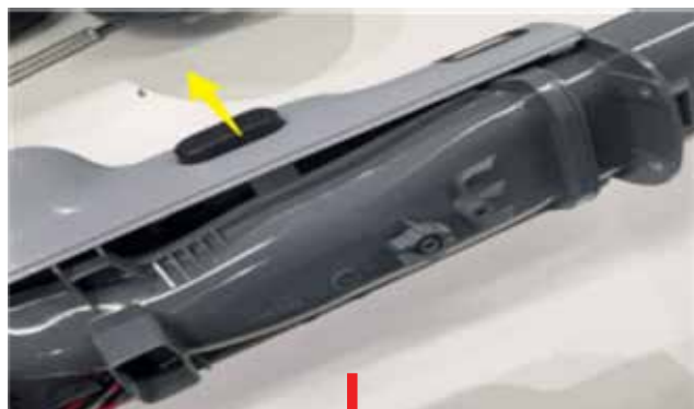
23. Remove the container release button
