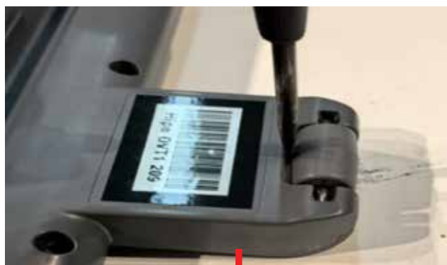
50. Release rear wheel and shaft
