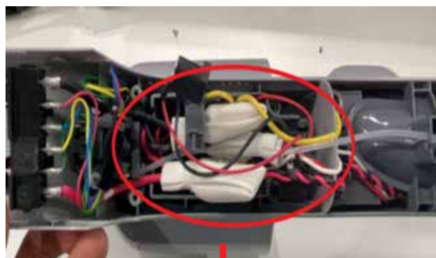
26. Pull the cable from the slots
