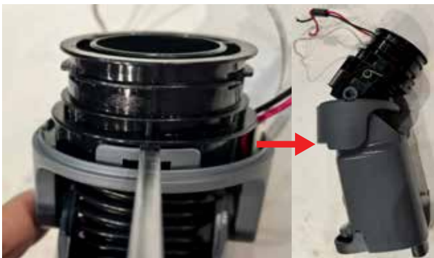
55. Push snaps in lower connector and then move the lower connector to upper connector
