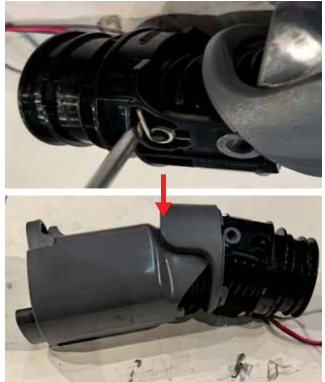
57. Release lower connector inside lining
