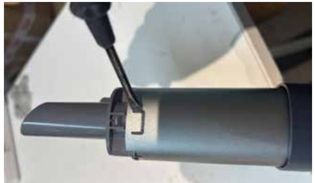
11. Pull telescope lower connector and telescope inner PP tube out
