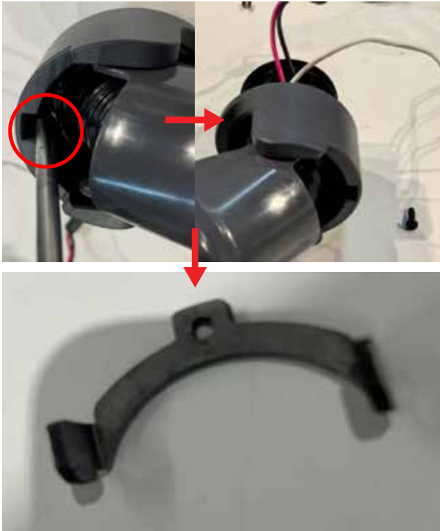
55. Push snaps in lower connector and then move the lower connector to upper connector
